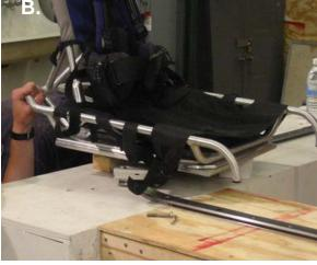
Figure 10.2. A. Seat Plate and Trolley Sliding along Curved Track Section. B. Seat Assembled to Trolley.
